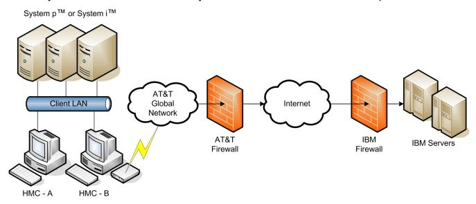
In this scenario the HMC uses one of the configured phone numbers to dial the modem, connecting to the AT&T Global Network. After the modem connects the HMC authenticates itself and establishes a Point-to-Point Protocol (PPP) session between the two modems. Finally, after the PPP session has finished, AT&T allows IP connections through a "Fenced Internet," which completes the network between the HMC and the IBM servers.
