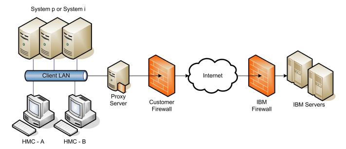
To forward SSL sockets, the proxy server must support the basic proxy header functions (as described in RFC #2616) and the CONNECT method. Optionally, basic proxy authentication (RFC #2617) may be configured so that the HMC authenticates before attempting to forward sockets through the proxy server.
