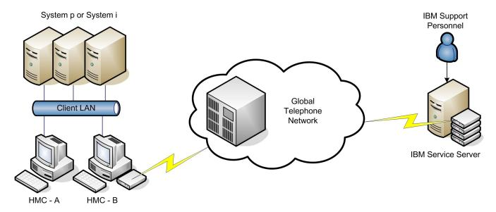
For remote service over a modem, the modem must be set up to accept incoming phone calls. An IBM representative then logs into a special server and uses that to dial directly into the client's modem. After the modem answers, a PPP session is initiated, and the IBM representative must authenticate using credentials based on the value the client entered into the **PPP address** field on the Customize Inbound Connectivity panel.
