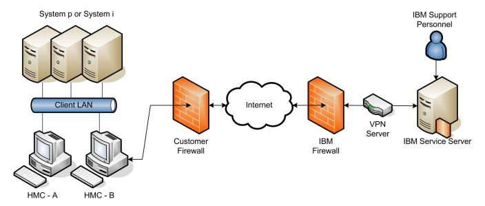
A remote service VPN session can be initiated over a modem, Internet VPN, or a pass-through i5/OS partition. At least one of these methods of connectivity must be configured through the Outbound Connectivity panel.
