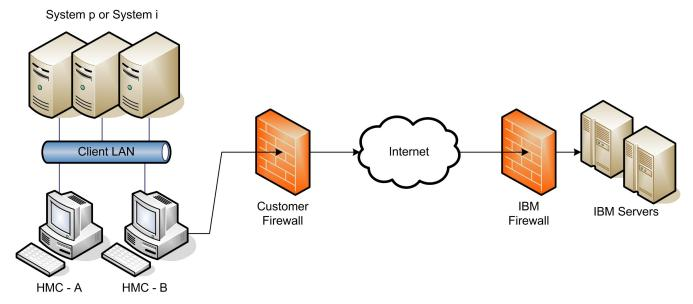
In this setup the HMC connects through the client-provided Internet connection by the default route. For this type of configuration the client can optionally use a second network card to physically separate the local system network from the Internet-enabled network.
